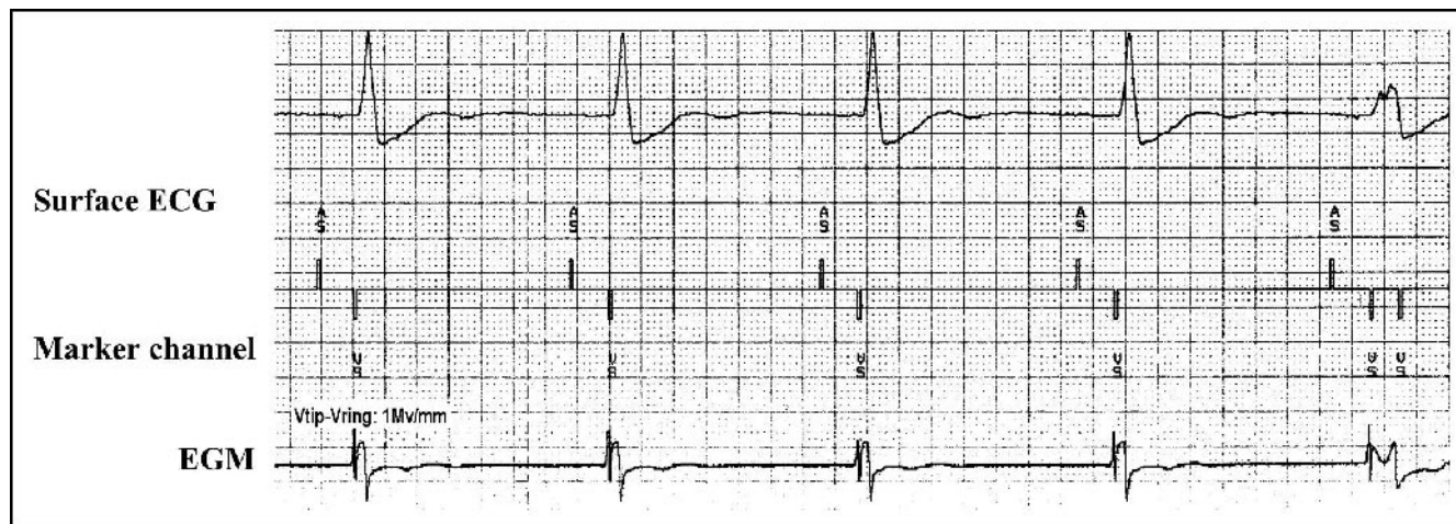
Figure 12. Ventricular oversensing due to conduction delay of last beat with LBBB. Notice much wider EGM on last beat
